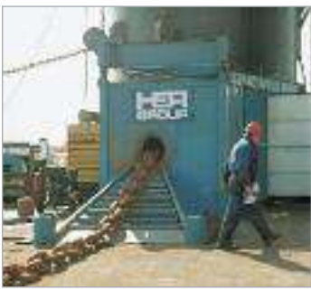
PE4004S pump and RD3006 cylinder used in a special press which repairs damaged chain links for the shipping industry.
