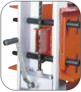
Lifting screw and locking pins make bolster raising a one-man job.
